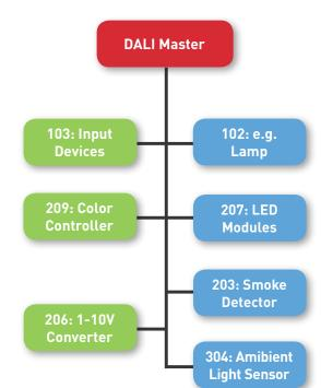
On the hardware side, Nuvoton offers two specific device series for DALI-2 devices namely NDA102 (for control gear) and NDA103 (for control/input devices).
