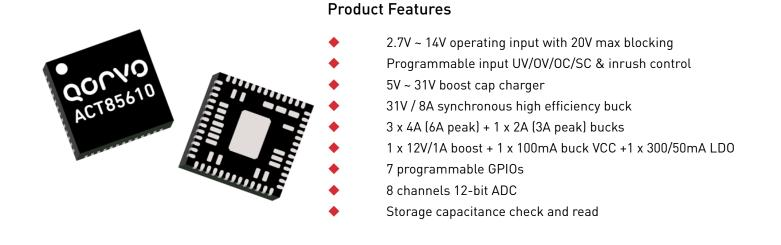
The ACT85610 device is a highly integrated, high configurable multiple output power management unit (PMU) with builtin power loss protection (PLP) IC. There are four high efficiency Bucks that can supply 3 x 4A and 1 x 2A current with the output as low as 0.6V. In addition, there is a Boost regulator with 12V output and a fixed output Buck to provide the power for IC itself and to supply power to the gate drivers in regulators for maximum efficiency
