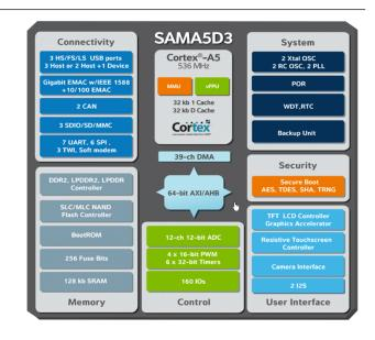
BGA324 (15x15 in 0.8pitch) package and also a small package option BGA (12x12mm in 0.5 pitch)
