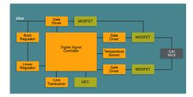
Wireless charging works by transferring energy from the charger to a receiver via electromagnetic induction. The charger uses an induction coil to create an alternating electromagnetic field, which the receiver coil converts back into electricity to be fed into a battery or directly to an application. Typically, the charger and receiver should be close and correctly aligned over the top of each other, although a set orientation is normally not necessary.
