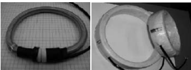
Figure 4.a Figure 4 Figure 4.b (Figure 4.a Flexible Coil, 4.b Rigid Coil.)
